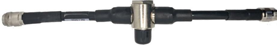
The 10332ZA phasing harness is a two-way cable power divider intended for the coupling of two UHF side mount dipoles. This Phasing Harness comes with a female input connector and two female output connectors. It affords a wide bandwidth, matching that of the two-stack array.
